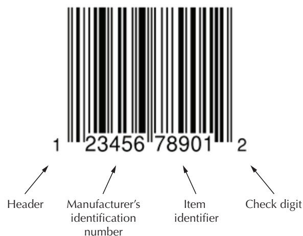
Figure 3: Anatomy of a Bar Code
